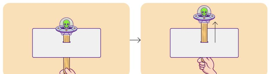
Door bolts and drawers use slider mechanisms.
