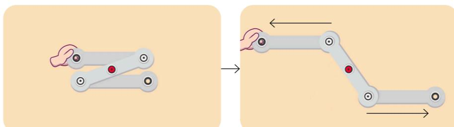
Toolboxes and scissor lifts use linkage mechanisms.
