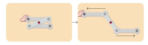
Toolboxes and scissor lifts use linkage mechanisms.
